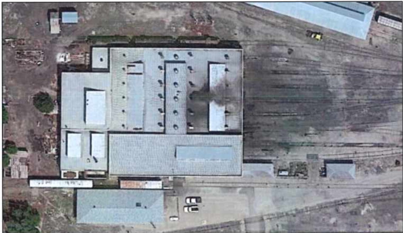
Photo 2 – This is an aerial view of the engine house/machine shop roof. This is the largest building on the complex. The roof area covers approximately 36,000 square feet. The engine house/machine shop building does not have a single roof, rather it has fourteen different roof levels with a mixture of roofing surfaces. In addition to repairing the roof itself, some of the parapet walls that separate the different levels are crumbling and need repairing too. A plume of smoke can be coming out of the one of the smoke jacks.
